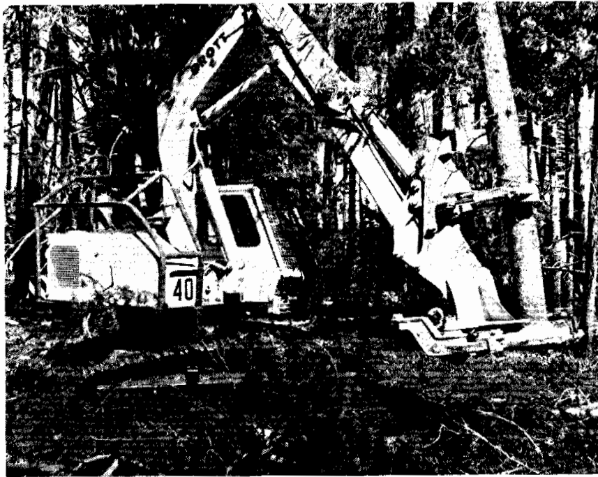
Figure 4.--A feller-buncher was employed on the Teton site to fell and bunch whole trees on the intensive utilization units.
